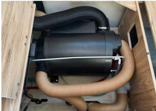
*Allows air in and burnt gas out.*
