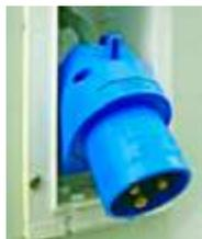
The connection to the mains is done by means of a cable that can be plugged in outside the motorhome to the blue P17 outlet. It is located either on the vehicle's exterior panels or in the service compartment which is accessed through a hatch.
